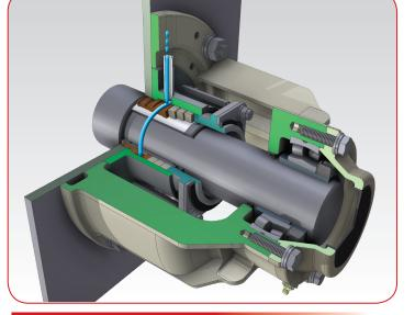
SECTION OF SHAFT AND SEAL
